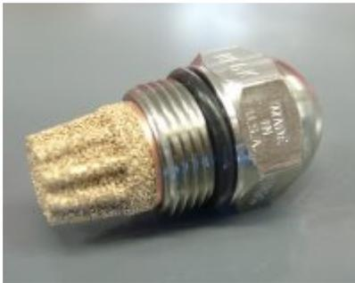
Nozzles over time do need cleaning or worst case - replacing. The time in-between cleaning or replacing nozzles can depend on water quality as discussed above. As seen in the picture to the left each nozzle has its own filter that stops small debris from entering the nozzle and clogging the orifice.
