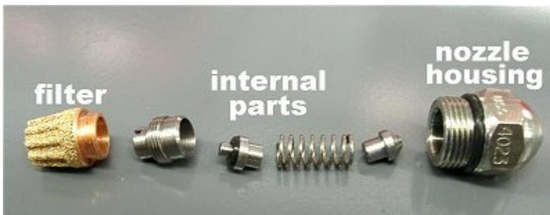
Cleaning the Hago 4023 nozzle can be accomplished a number of different ways. The most common way to clean nozzles is to disassemble the nozzle and blow the housing out with compressed air.
